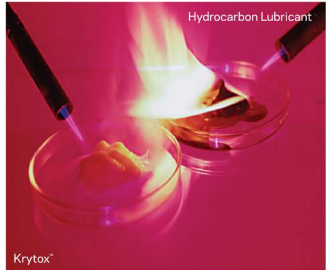
Hydrocarbon-based lubricants burn; Krytox ™ does not.
